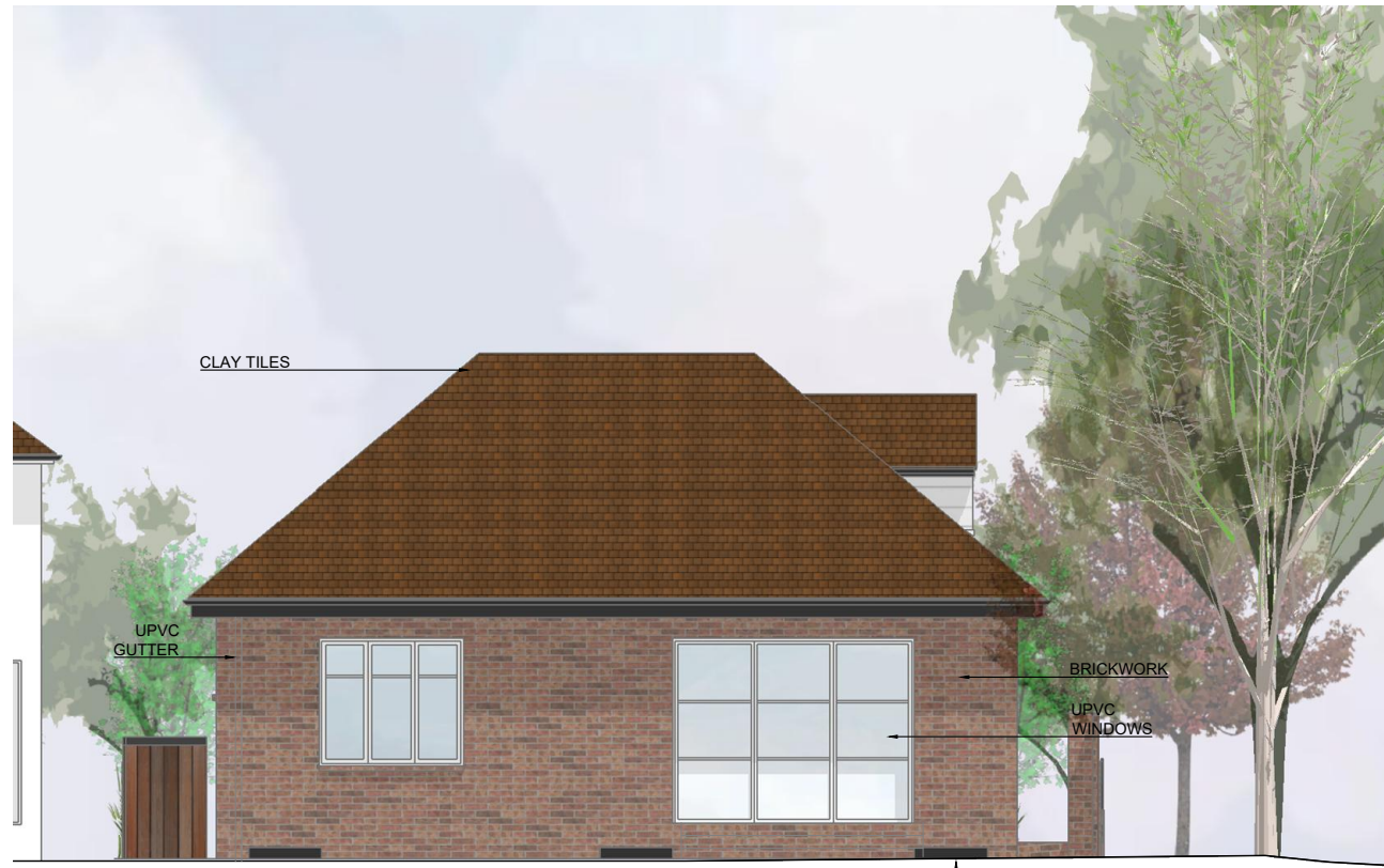
HOUSE A PROPOSED EAST ELEVATION Scale 1:100
