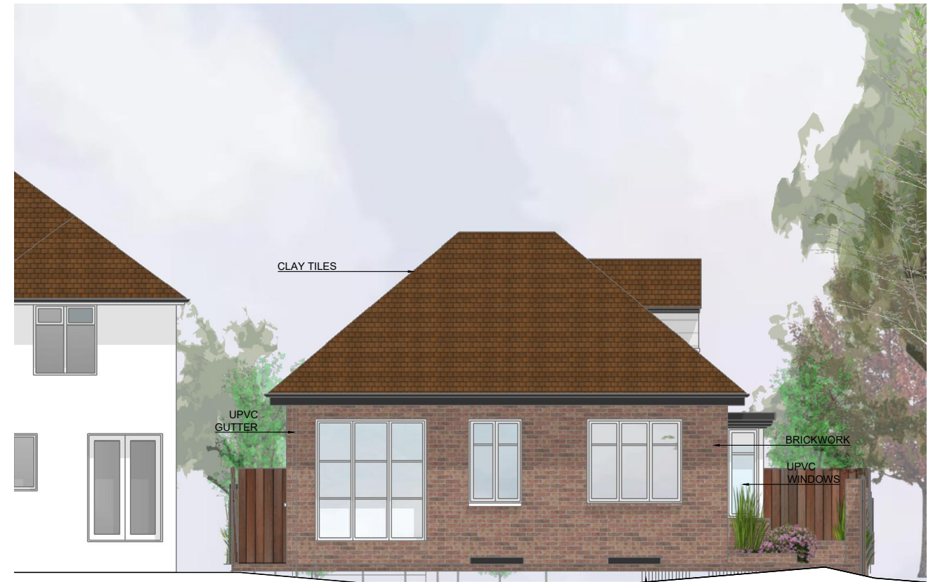
HOUSE B PROPOSED EAST ELEVATION Scale 1:100
