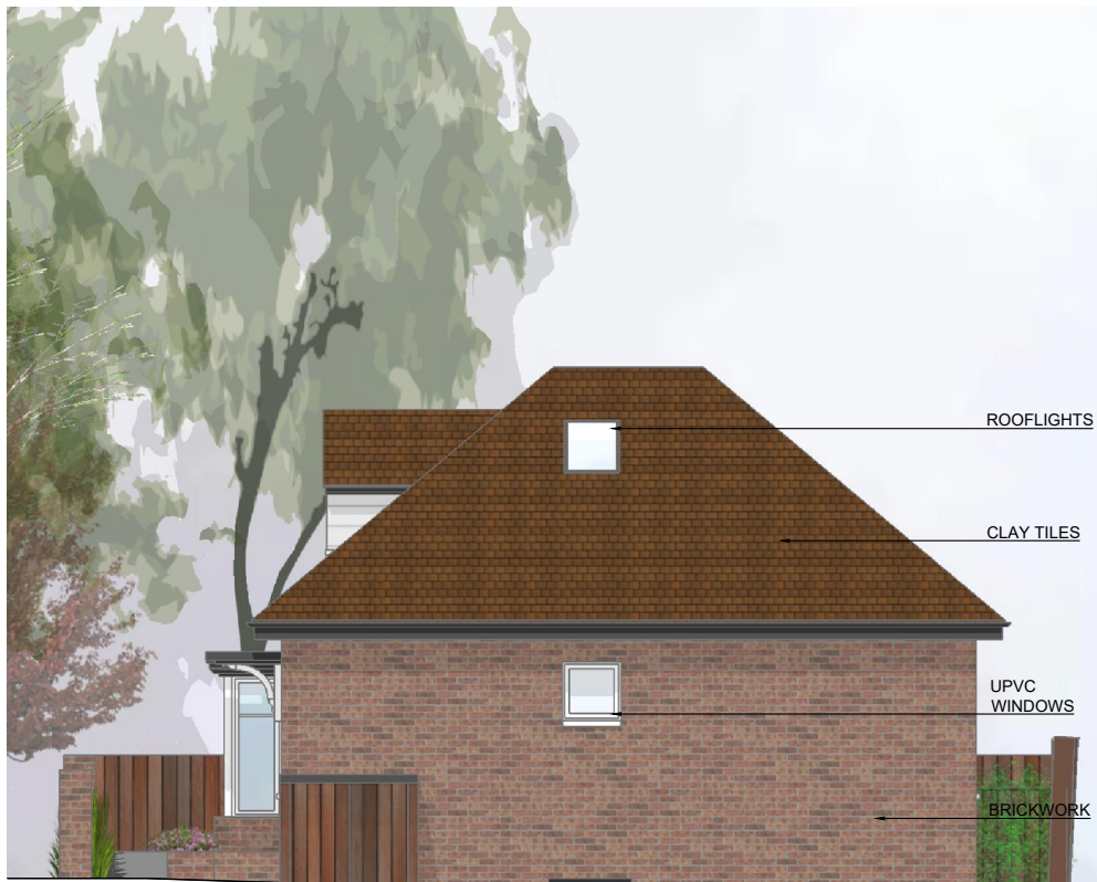
HOUSE B PROPOSED WEST ELEVATION Scale 1:100
